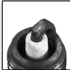
Spark plug has dry deposits
